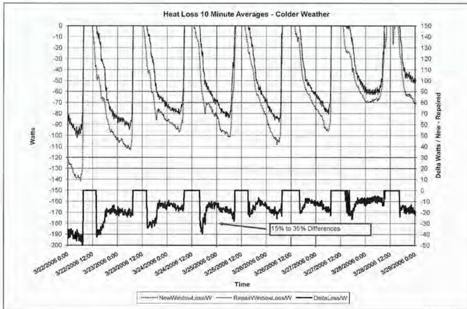
Fig. 12. Heat loss during the coldest week.
