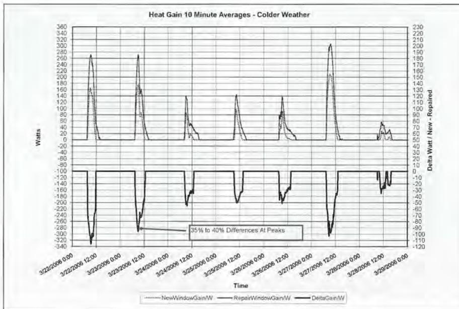
Fig. 10. Heat gain during the coldest week.
