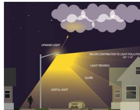
Figure 205.1: Light in the Nighttime Environment The principles of DarkSky International should also be considered while designing roadway lighting: all lighting should be useful, be targeted where it is needed, only be as much light as necessary, and should be controlled.
