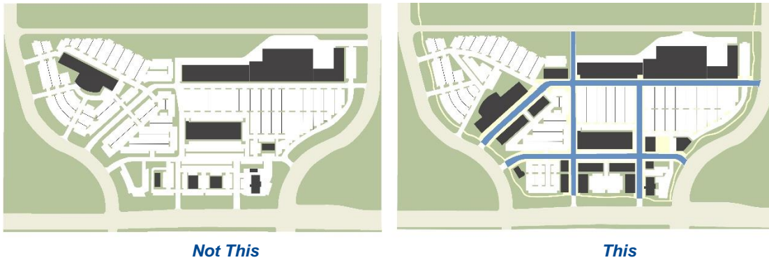
Figure 24-7-1: Internal access streets.
