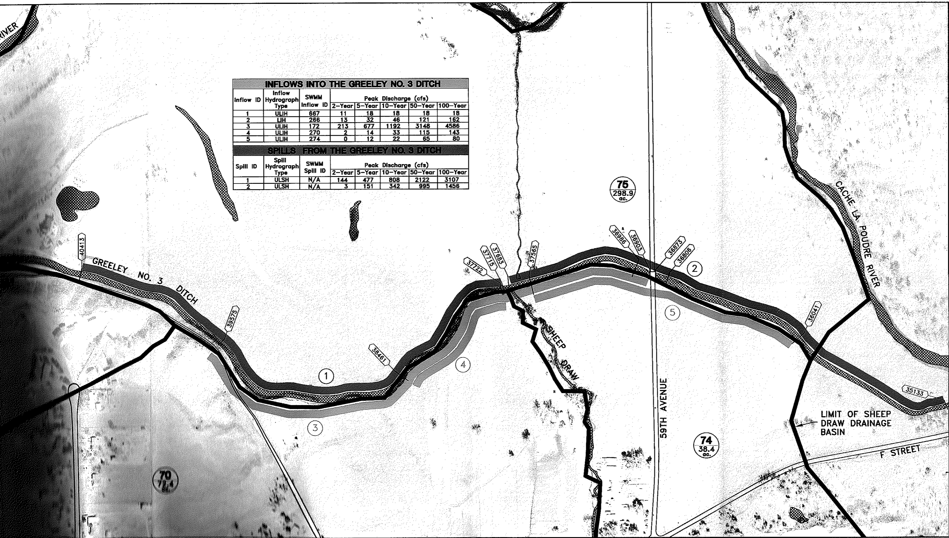
SHEEP DRAW BASIN-EXISTING CONDITON INFLOW HYDROGRAPH, LATERAL SPILL LOCATION (HEC-RAS UNSTEADY FLOW ANALYSIS), AND CROSS SECTION IDENTIFICATION MAP
